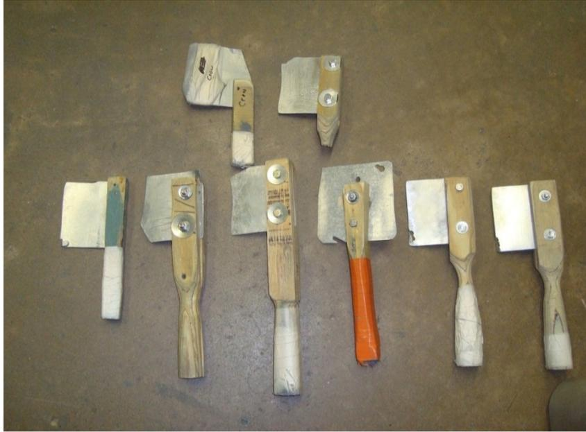
**Figure 7: Hatchets used to remove paint.**
