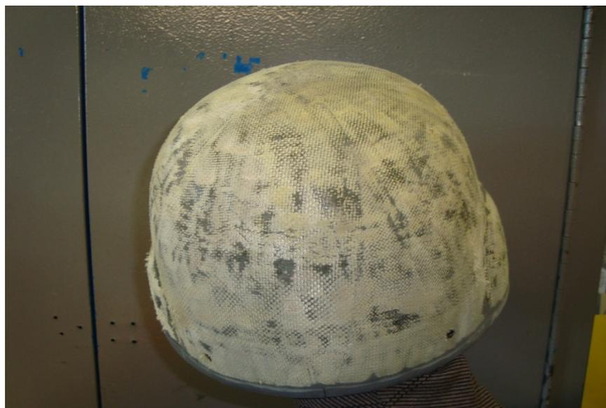
**Figure 9: Damaged ACH after paint removal.**
