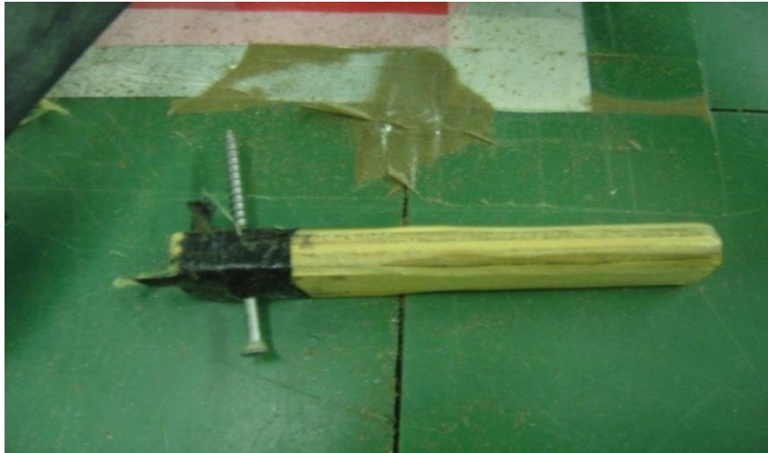
**Figure 8: "Screw tool" used to strip Kevlar**
